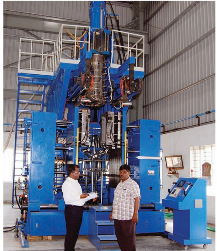
Blow molding machinery to manufacture HDPE Float and covers for Paddle wheel Aerators imported from Cheway machinery, Taiwan
