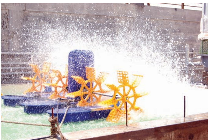
Aerator with four paddle at Nandini's aerator testing facility
