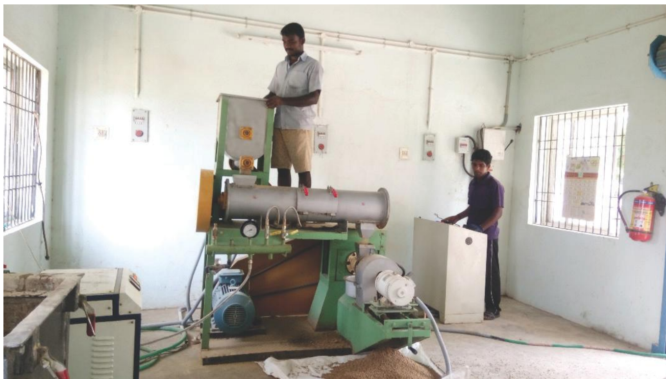
Fig. 5: Production of tilapia floating feed using single screw extruder
