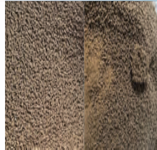
Pellet with ARMOUR (PDI 96%) vs Pellet without ARMOUR (PDI 70%)
