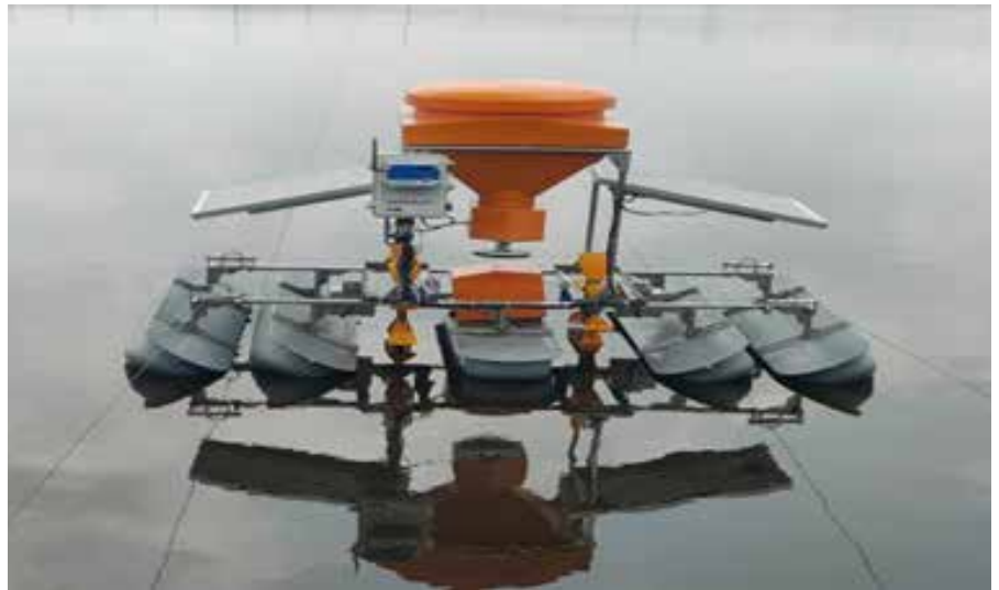
Floating IoT feeding and propulsion device on shrimp pond
